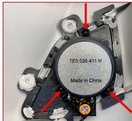
**△ Pro tip:** We recommend covering the area behind the loudspeaker with an insulating mat to reduce resonance. Ask your dealer for EMPHASER EM-DM2 - this mat is a combination of alubutyl and open-pored foam and perfectly suitable for the intended use.
