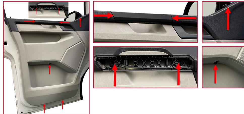
To remove the rivets, use a metal drill with a diameter of 7.5 mm or larger and carefully drill the rivet head. Take out the speaker and remove the remains of the rivets with a 9 mm nut and a pipe wrench: Hold the 9mm nut behind the rivet. One cheek of the pipe wrench rests on the 9 mm nut, the other cheek on the rivet. Squeeze the pipe wrench; the rivet is caught by the nut and the sheet metal remains undamaged.
